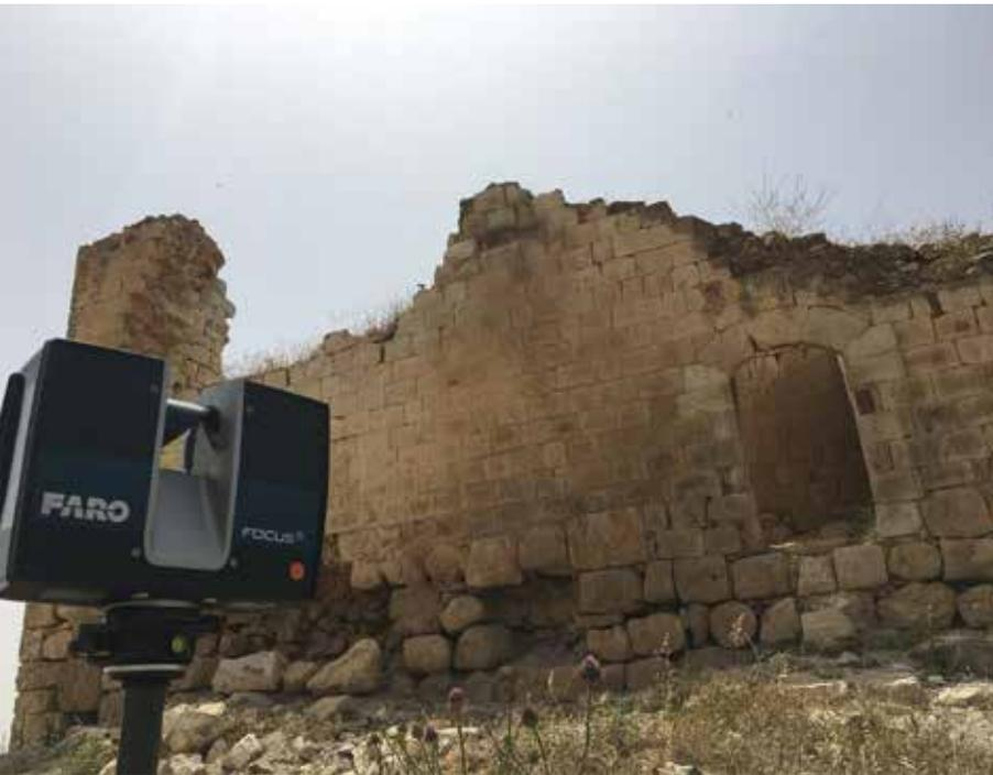
■ One of the best ways to capture with utmost detail the true environment of a heritage site is through a 3-D laser scanner, shown above.
